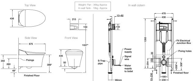
\* Nominal dimensions based on in-wall tank being installed at designated height. This height can be adjusted to suit user preference.
